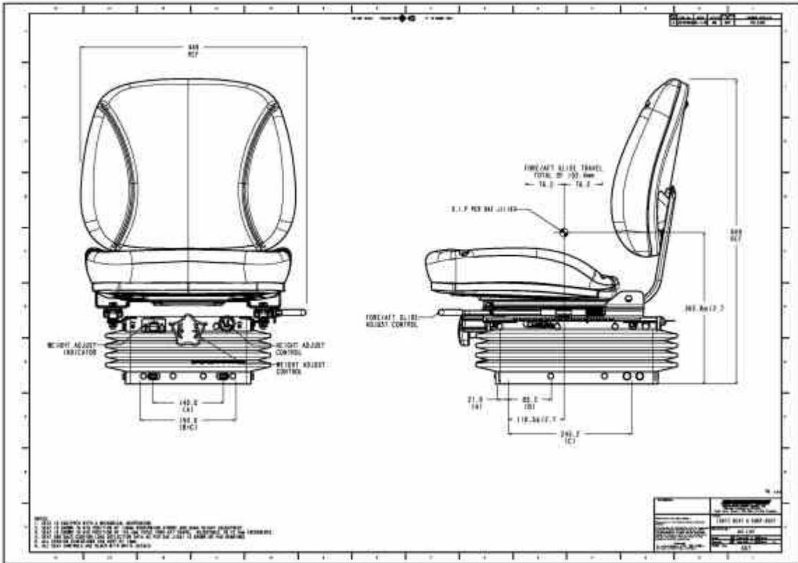
Medium mechanical scissor suspension with integrated height adjustment & damper
